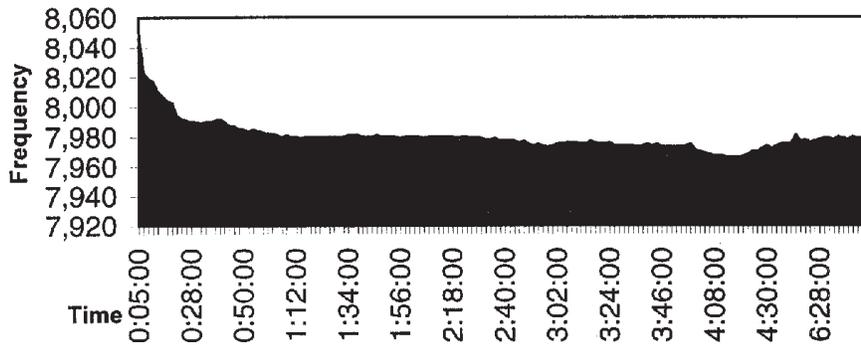
**Graph B-1:** Only the last 4 digits of the frequency output are displayed. The table shows the results of the 24,997,980 MHz crystal in normal time and space, over eight hours.
